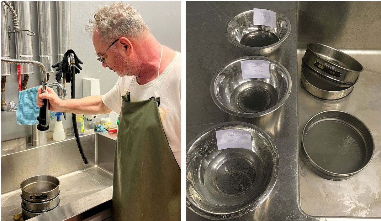
Fig. 10 Washing disintegrated sediment over a sieve stack with 250, 125 and 63 \mu\text{m} . The residues are then gently washed into stainless bowls
